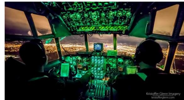
During Daylight hours, crews fly sorties under VFR conditions at altitudes ranging from 300 feet AGL to 500 feet AGL at speeds averaging 210 KIAS (Approximately 242 MPH).
